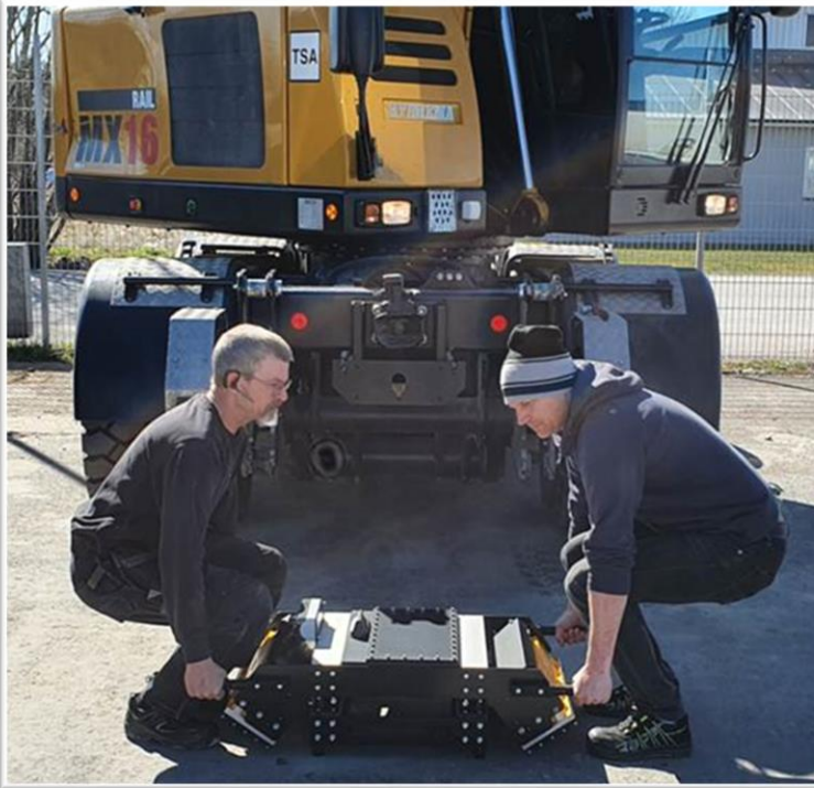
Step 1, Lift LTM to pre-assembled bracket
